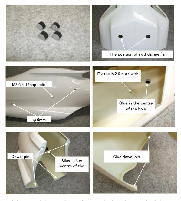
•Dowel pins are attached temporarily, so make sure to glue them using epoxy glue. (x4)
