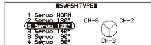
⑫ Input the numbers, +/- and REVERSE the direction of each servo as shown in the figure.
