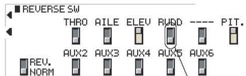
※NOTE the rudder direction will depend on the gyro and rudder servo used. Please check carefully.
