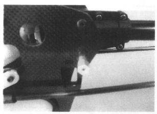
2To fix the 18.5 mm cross-member with a 3 x 15 set-screw.
