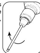
**5. Inserting the starter shaft**
