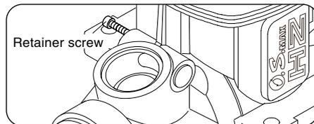
2. Insert the carburetor rubber gasket on the carburetor body securely. Then, insert the carburetor in the crankcase.
