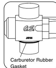
**Note: In case it is hard to insert the carburetor in the crankcase. Do not force it, or damage to the crankcase can occur.**
