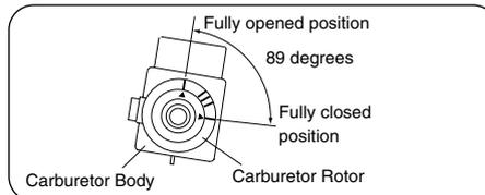
When the triangle mark on the carburetor rotor meets the far right mark, the throttle is fully closed. When the triangle mark meets the top mark, the throttle is fully open. The range is 89 degrees. You may use the other three marks as the reference marking of throttle opening to your preference when hovering.
