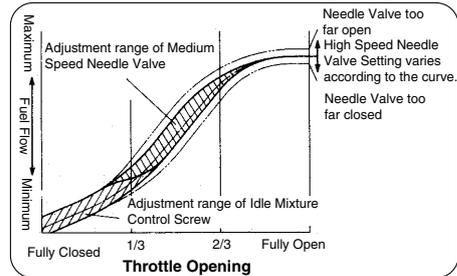
**NOTE: With this carburetor, neither the Idle Mixture Control Screw adjustment, nor the Medium Speed Needle Valve adjustment will have any effect on mixture strength when the throttle is fully (or almost fully) open.**
