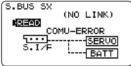
④ Connect a S.BUS servo to set up.
