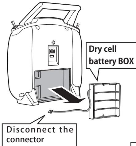
Refer to the previous description and remove the transmitter battery cover. After removing the dry cell battery box from the transmitter, disconnect the connector.
