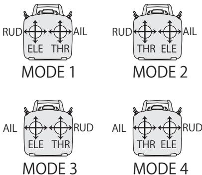
This is the MODE1 ~ MODE4 setting. The initial state is MODE2. To change the mode the stick ratchet must be changed. Request that this be done by Futaba Service. (Charged modification)
