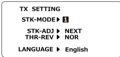
Turn on the power switch with the + key and – key pressed in the power off state. The screen shown at the left appears. To return to the home screen, turn off the power and then turn the power back on without pressing the keys.
