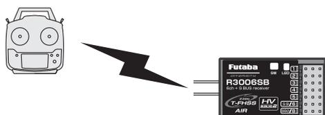
7. Immediately **turn on the receiver** power. The receiver will enter the linking state (**LED blinks red**) about 3 seconds after the receiver power is turned on.
