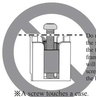
Do not loosen the screw past the top of the frame, as this will cause the screw to rub on the back case.
