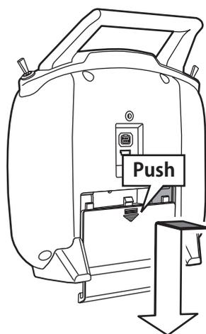
Slide the battery cover off the transmitter in the direction of the arrow in the figure.
