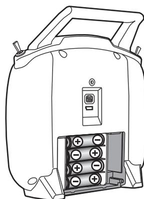
Load the new AA size batteries. Pay very close attention to the polarity markings and reinsert accordingly.
