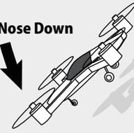
**Front slide** ← **Elevator stick DOWN (moved to the top)**
