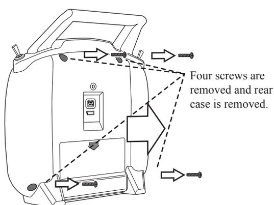
Four screws are removed and rear case is removed.
