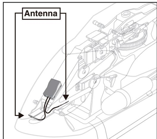
\*The two antennas should be placed at 90 degrees to each other.
