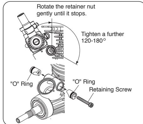
1. Loosen the retainer screw, rotate the carburetor to its correct position and make sure that it is pressed well down into the intake boss, compressing the rubber gasket, before retightening screw.
