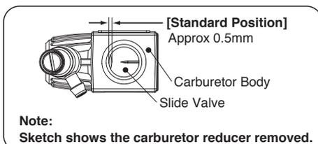
**NOTE:** While the Mixture Control Valve and the Metering Valve are set at the standard position when the engine leaves the factory, readjustment may be necessary, occasionally to allow for changes in fuel formula and climatic conditions. Readjust the controls only when satisfactory results cannot be obtained with the standard positions following the instructions mentioned in the "CARBURETOR ADJUSTMENT" section.
