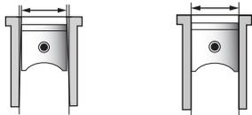
When the engine is cold. When the engine is hot.
